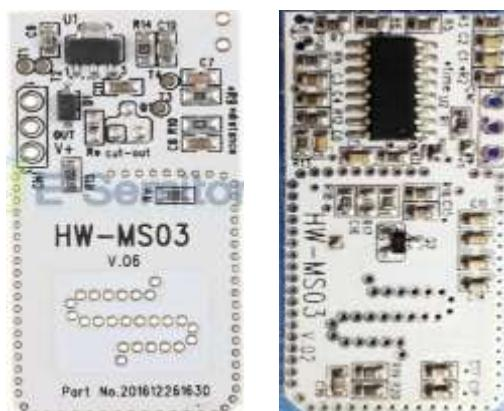
**Figure 2** Microwave sensor HW MS03
