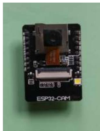
**Figure 3** The photo of ESP32\_CAM
