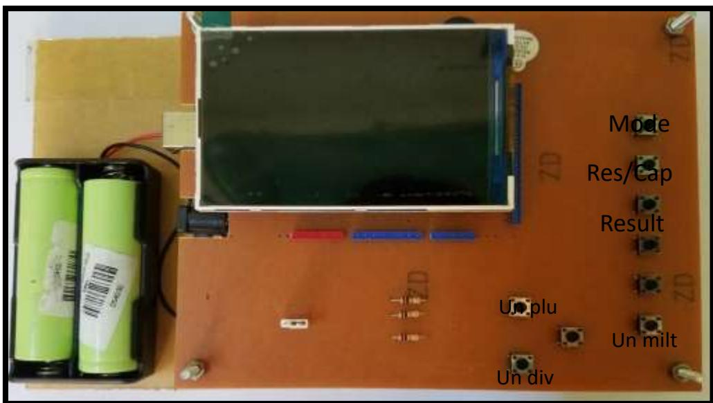
**Figure 8** The teaching aid for astable and monostable circuit
