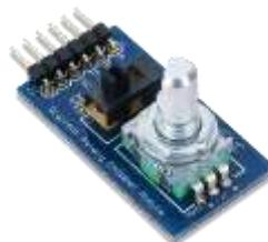
**Figure 2** Component of rotary encoder module
