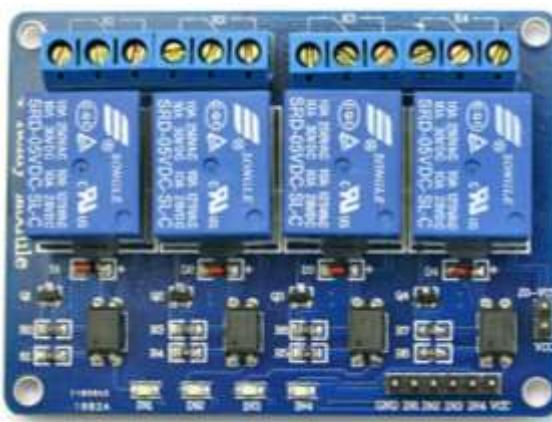
**Figure 3** 4-channel relay
