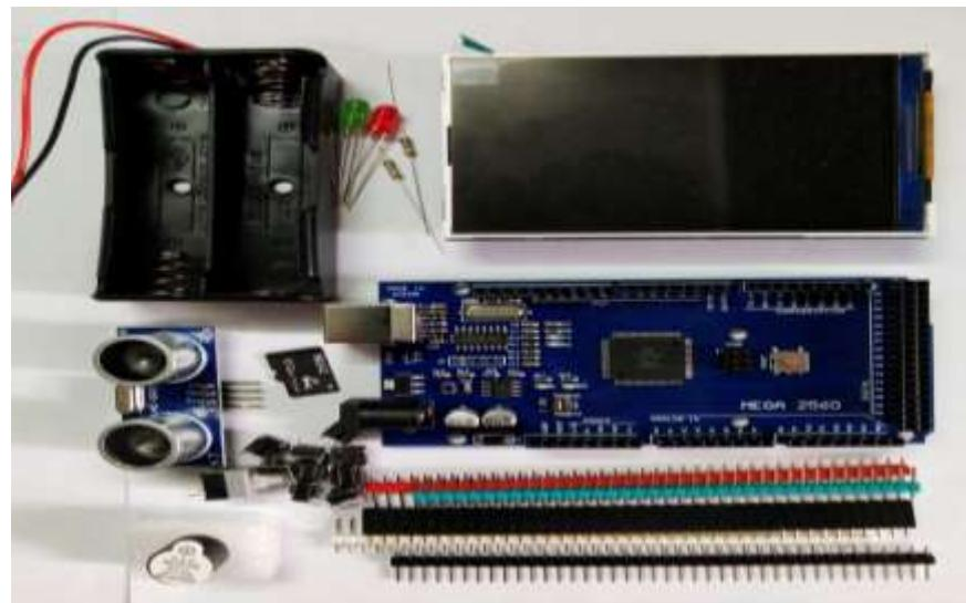
**Figure 2** Components of electronic ballot for general election
