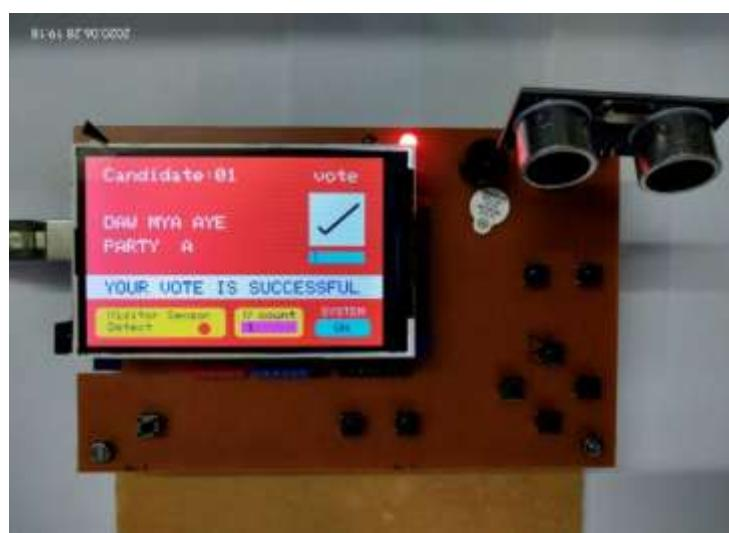
**Figure 9** The LCD display after voting successful
