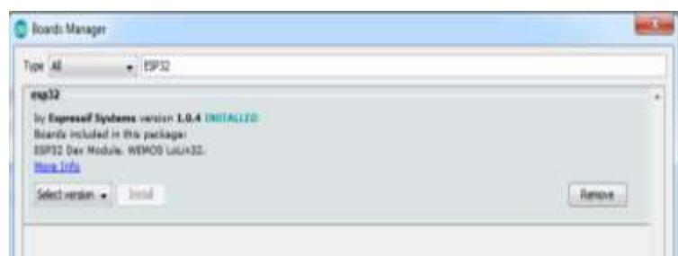
**Figure 7** Installing ESP32
