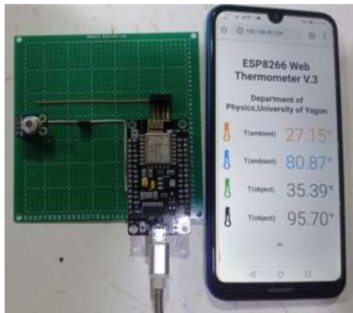
**Figure 7** Contactless thermometer
