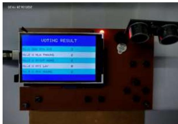
**Figure 10** The LCD display for voting results
