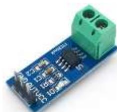
**Figure 5** Component of current sensor module
